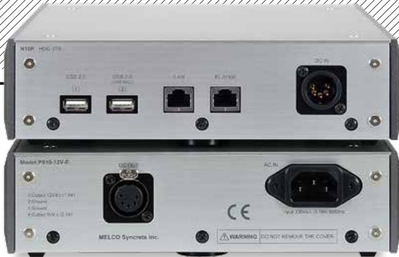
**ABOVE:** Melco offers network and direct player Ethernet connections from the player [upper] plus two USB-A ports, one to drive a USB DAC and one to connect an (expansion) USB HDD. The 5-pin XLR carries 5/12V DC from the PSU [lower]
